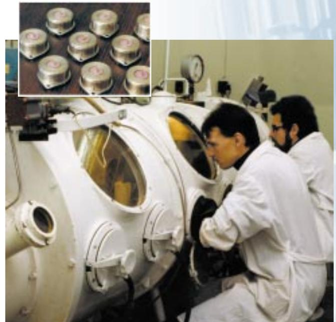
VNIIEF specialists assembling batteries in inert gas chamber
