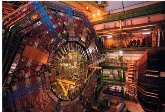
The Compact Muon Solenoid (CMS) experiment is one of two large particle detectors built on the LHC
