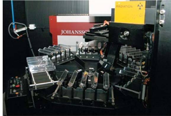
Russian made scintillating crystals used in the CMS detectors
