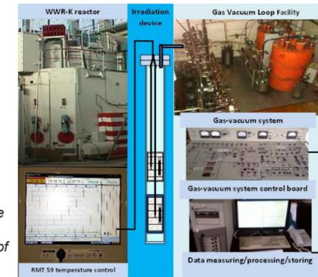
The general scheme of the equipment used for irradiation of SiC specimens
