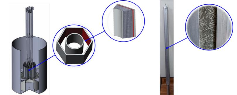
The structure of the new type reflector element
