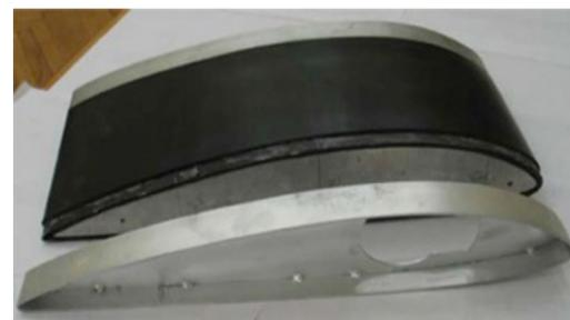
VGR Blade Rib and Blade Section with Flexible Element
