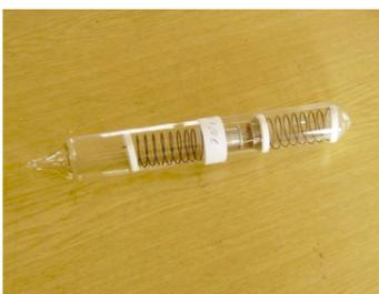
The new cathode in a transporting ampoule
