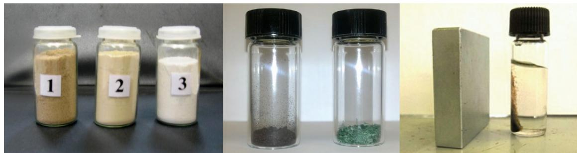
Samples of pectin-based nanoformulations: a set of purified native pectin samples, Cu (o) nanocomposite, Cu (II) complex, magnet liquid Fe<sub>3</sub>O<sub>4</sub>-Pec (from left to right)
