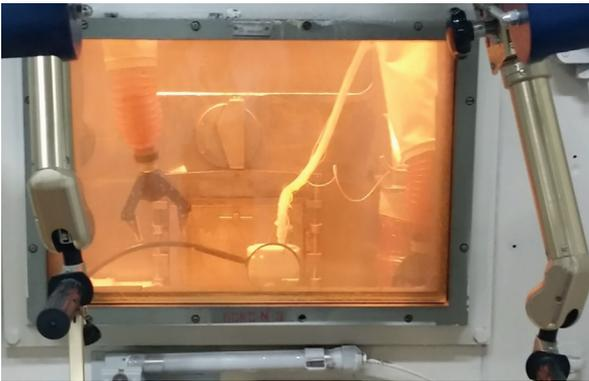
“Hot” cell with device for the electric dissociation and acid leaching of irradiated fuel specimens.
