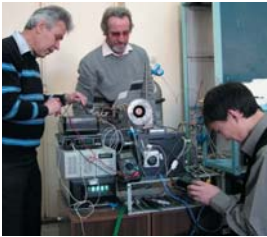
Laboratory tests of the prototype Power Plant working on methanol with 150 W capacity
